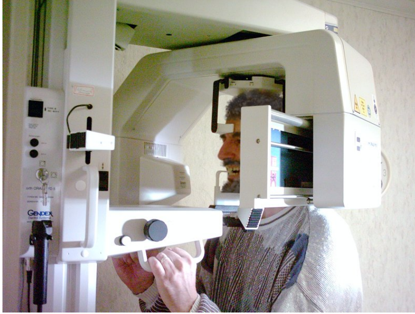
Figure 1.3: A panoramic radiography machine also called panoramic unit. During the image acquisition, the patient stays in the center of rotation of the X-emitter and receptor. Both rotates in tandem to generate the dental panoramic radiograph (Wikipedia contributors, 2024).
