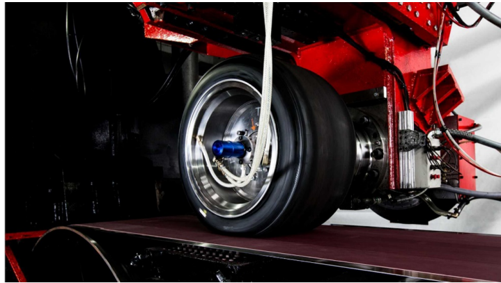
Figura 4.3: "Flat-track" para teste de pneus. Fonte: https://calspan.com/automotive/tire-performance-testing/motorsports-tire-testing
