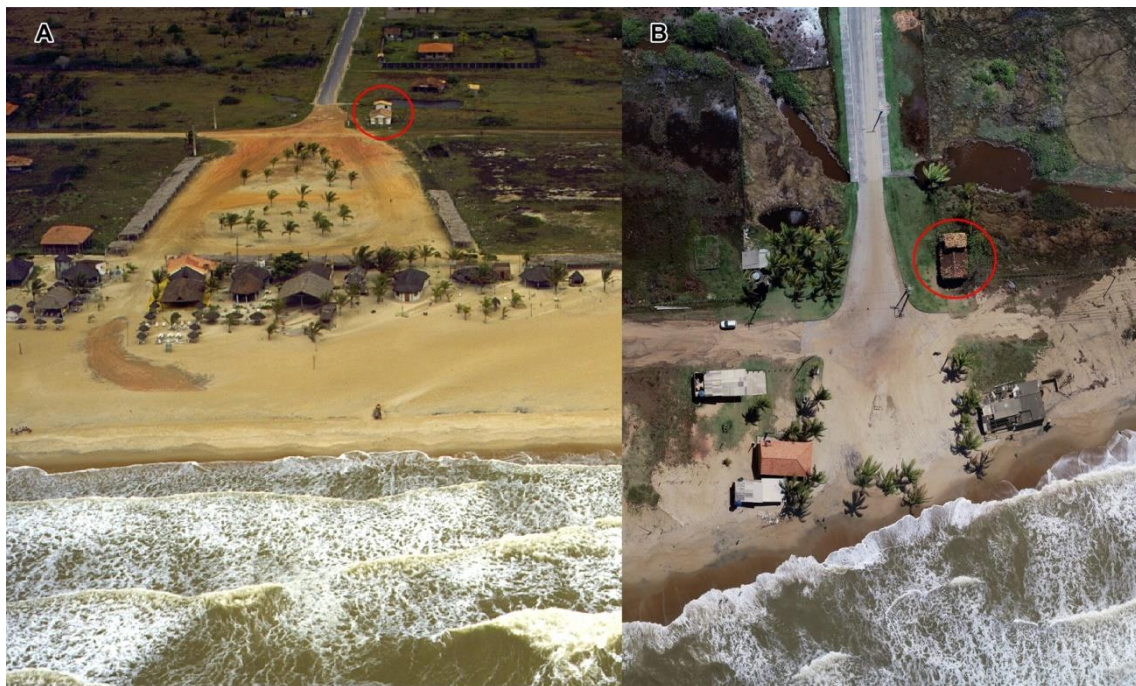
Figure 9: Erosion in the vicinity of the mouth of the Jequitinhonha River. A. Oblique photograph of Belmonte beach in 2003; B. Vertical photograph of the beach from the same location in Belmonte in the year 2022. The red circle indicates a common element in the two photographs.
