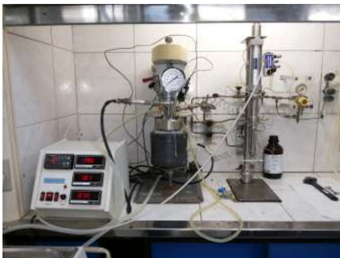
Figure 3.1 - Polymerization system for HDPE production.
