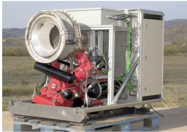
(b) UCP com receptor DIR e a motor Stirling SOLO 161
