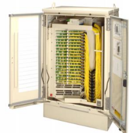
08 - OUTDOOR FDH 3000 ME- DIUM (COM 4 BANDEJA EMENDA, 1 BANDEJA C/ 64 ADAPTADORES SC-APC, 1 SPLITTER 1X64 NC/SC-APC)
