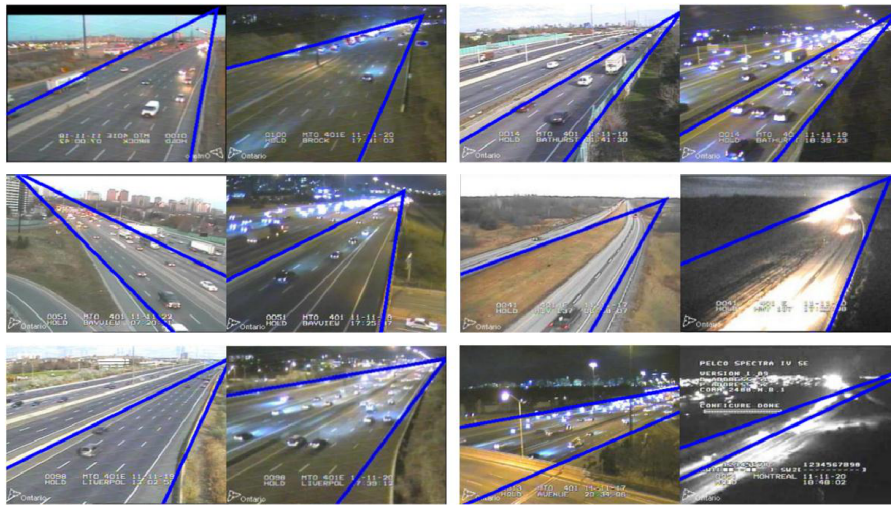
Figure 2.22: Examples of road borders detection by the method of [Helala et al. 2012]. Images adapted from ibid.
