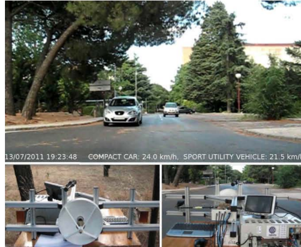
Figure 2.2: Interferometric radar at field experiments. The device is used to detect road lanes in order to support a traffic flow analysis process. Image taken from [Felguera-Martin et al. 2012].
