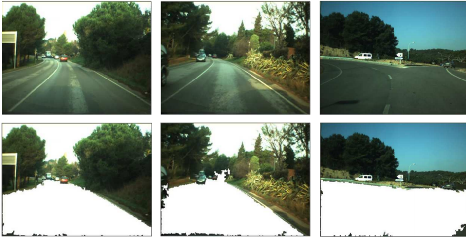
Figure 2.9: Examples of road segmentation produced by [Alvarez et al. 2008]. First row, input images; second row, segmented roads. Images taken from ibid.
