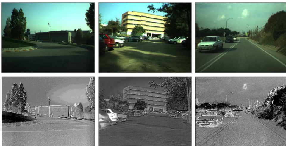
Figure 2.8: Examples of illuminant invariant images. First row, input images; second row, generated illuminant invariant models. Images taken from [Alvarez et al. 2008].
