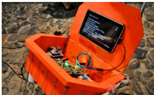
Figure 1: Sensorium device: arduino, sensors and tablet
