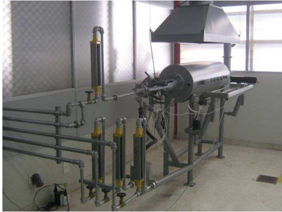
(a) View of Combustion Chamber and Rotameters. measurement.
