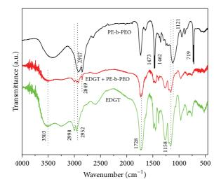
FIGURE 4: FTIR spectrum of pristine PE-b-PEO and electrospun fibers of Eudragit L-100 (EDGT) and Eudragit L-100 + PE-b-PEO (EDGT + PE-b-PEO).
