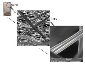
FIGURE 1: SEM images of electrospun fibers of Eudragit L-100.
