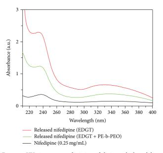
FIGURE 7: UV-vis spectrum of pristine nifedipine and released drug from electrospun fibers of Eudragit L-100 and Eudragit L-100 + PE-b-PEO.
