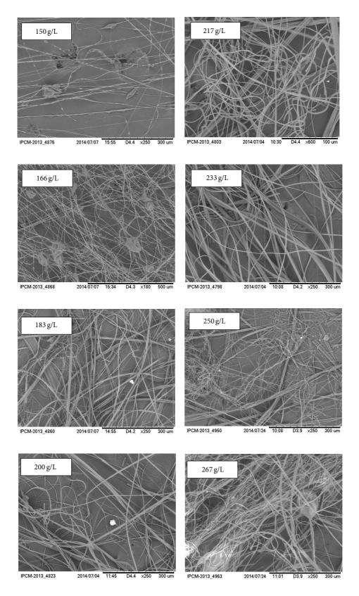
$FIGURE\ 2: Comparison\ of\ electrospun\ fibers\ of\ Eudragit\ L-100\ as\ a\ function\ of\ concentration\ of\ polymer\ (range\ of\ 150\ g/L\ to\ 267\ g/L).$
