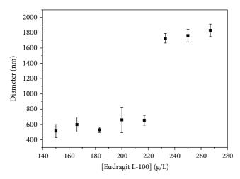
FIGURE 3: Dependence of diameter of electrospun fibers versus concentration of Eudragit L-100.
