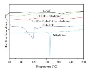
FIGURE 8: Comparison of DSC thermograms of Eudragit, PE-b-PEO, EDGT + nifedipine, EDGT + PE-b-PEO + nifedipine, and pristine nifedipine.
