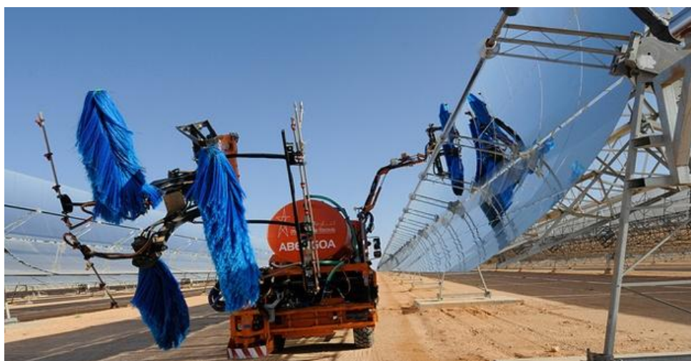
Fig. 20 Mirror cleaning adds to maintenance costs
