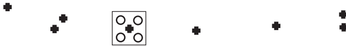
Fig. 4. Exemplary plan view of borehole (crosses) and foundation locations (e.g., quadruple shaft foundation for a bridge site); not to scale
