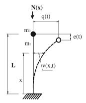
Fig. 1 Parameters for developing the mathematical model
