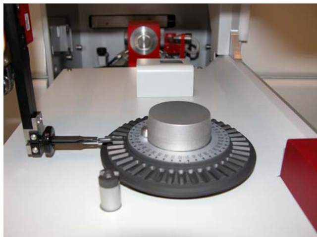
Fig. 2 Fully automatic accessory SSA 62 for automatic transfer of up to 62 SS platforms to a microbalance and into the graphite furnace. (Courtesy of Analytik Jena, Jena, Germany)
