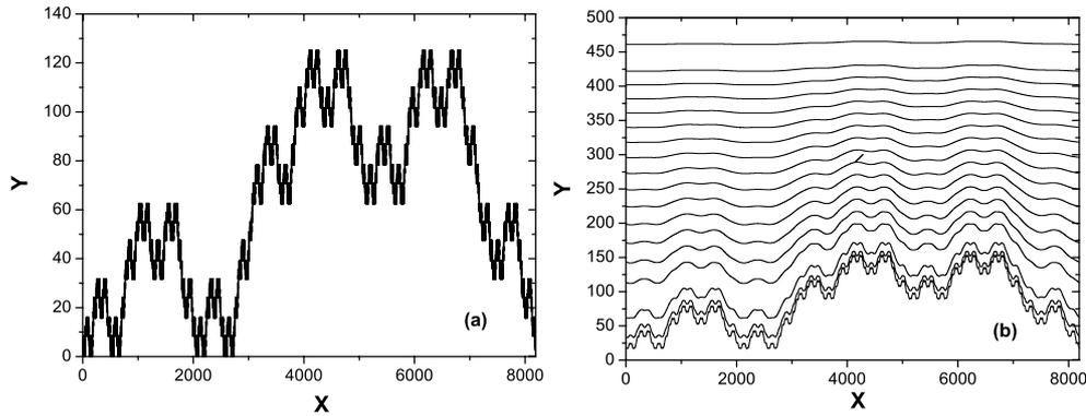
**Figure 1.** (a) Self-affine profile mimicking a rough boundary. (b) Equipotential lines  $\phi(x) = \phi_i$ ,  $\phi_i = 1, 7, 5n$ ,  $n = 2, \dots, 20$ , for the profile shown in (a).  $\phi = 100$  at the upper boundary is an approximation of  $\phi(y \rightarrow \infty) \rightarrow \infty$ .
