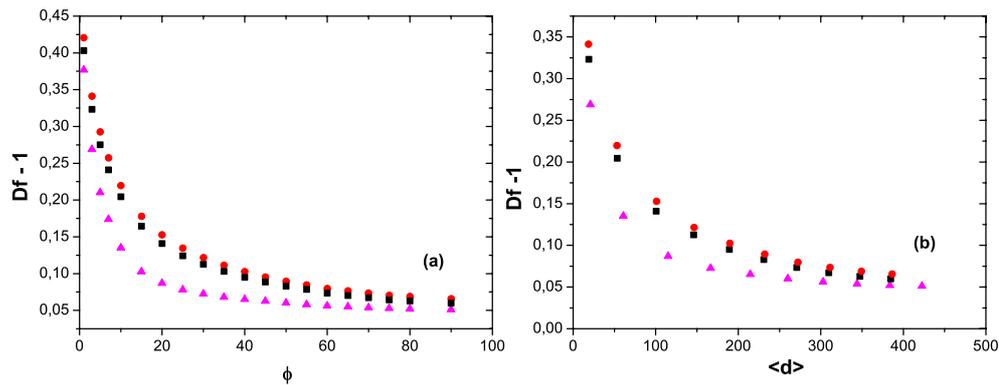
**Figure 3.** (a) Behaviour of  $D_f - 1$  as a function of the potential  $\phi$  for the three profiles. (b) Dependence of  $D_f - 1$  as a function of the average distance  $\langle d(\phi) \rangle$  with respect to  $\phi$ . Solid circles, squares and triangles indicate, respectively, profiles with 8192, 4096 and 2048 points.
