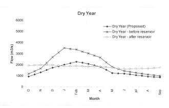
Figure 2 - Environmental flow hydrograms required for :(I) normal year and (II) dry year
