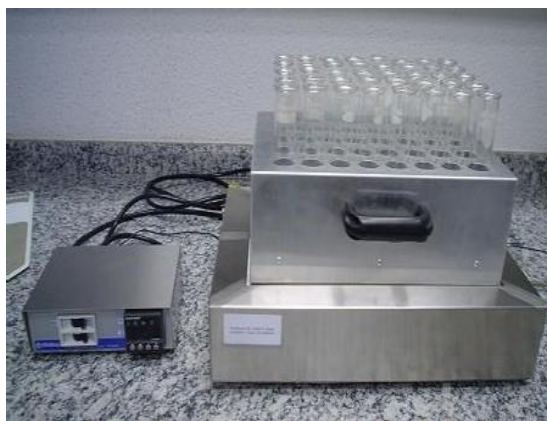
Figura 4. Bloco digestor TE-040/25
