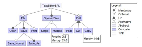
Figure 2.7: Feature Model of a Text Editor SPL.
