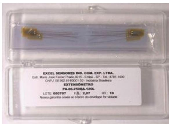
Figura 80 - *Strain gages* uniaxiais
